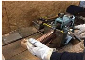
A swager tool is used to make the edge at the top – to stop the lid slipping off.
