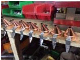
The first step is to cut all the parts out by using a 40 tonnes power press. This includes the nozzle, rim, body, bottom, air pipe and hinge. The lids are made first and the knob attached.
