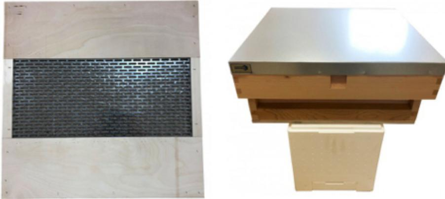
This excluder will hopefully alleviate some pressure. Made from a slotted steel excluder and 6mm birch ply with a 6mm bee space one side, flush on the other side, it will fit all BS nuc boxes including polystyrene. It enables a conventional super to be placed on top to give your bees that extra bit of room and curtail any swarming instinct. Lateral support may be required in an exposed position.
